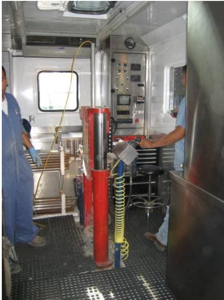
CPT Rig and Hydropunch sampling
